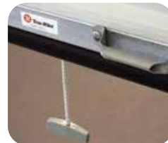
Sturdy galvalume bottom assembly is fitted with the Seal-Rite bulb and blade astragal for a protective weather seal. Zinc-plated exterior handle and molded plastic pull rope handle provide effortless opening and closing of the door.
